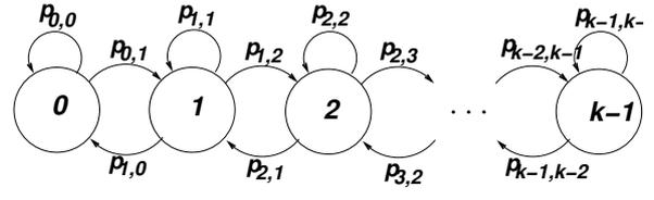
Fig. 2. Generic Model of the Wireless Channel
