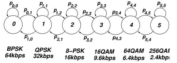
Fig. 4. A 6-state FSMC model of the Wireless Channel
