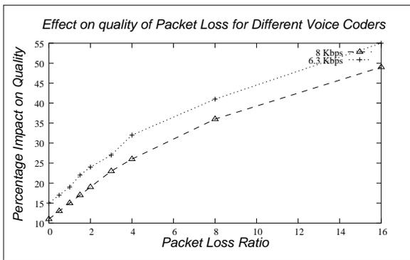
Fig. 1. Effect of Packet Loss on Quality for Two Voice Coders.
