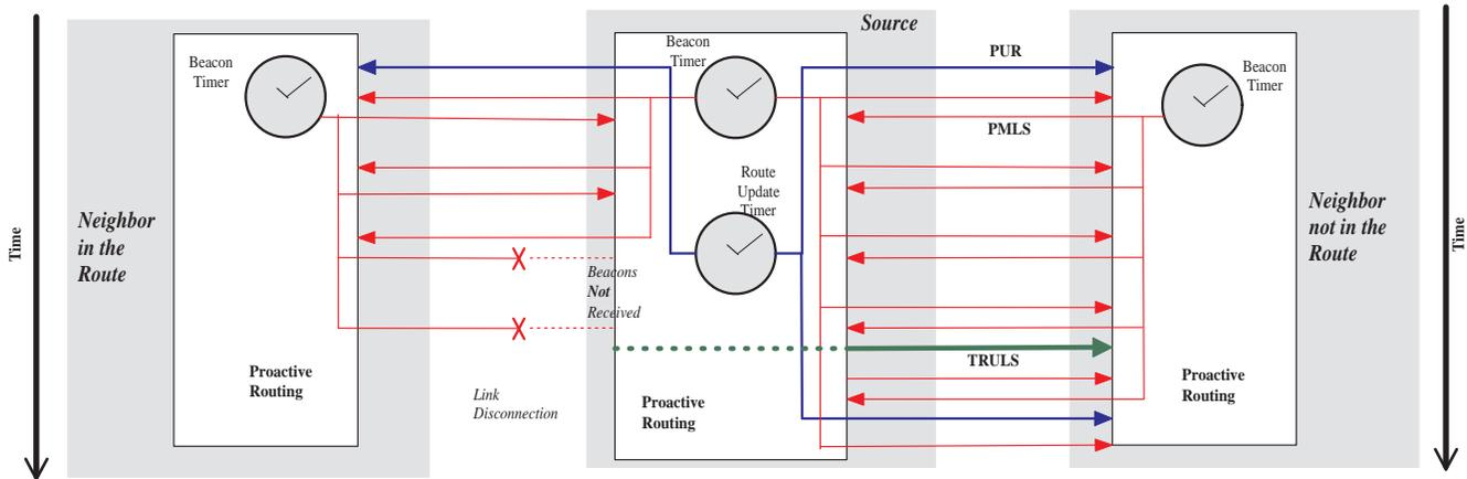
Figure 2: Periodic messages exchanged in proactive routing for MANETs
