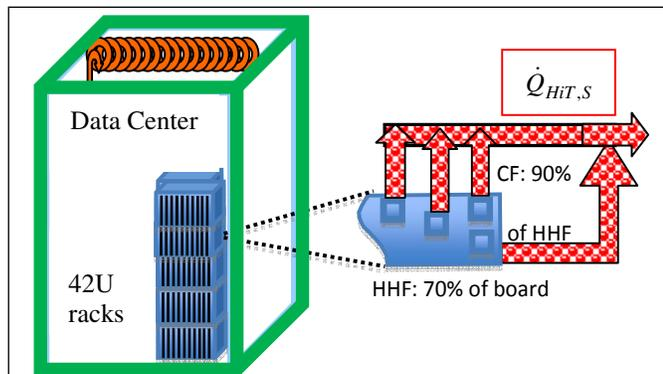
Figure 2. Detail view of heat capturing process from the server blades. A fraction of the heat from the hottest components on each blade is removed by liquid cooling to drive the LiBr absorption chiller.
