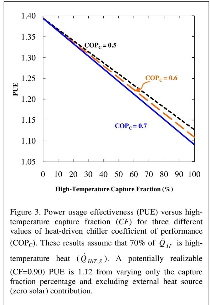
Figure 3. Power usage effectiveness (PUE) versus high-temperature capture fraction (CF) for three different values of heat-driven chiller coefficient of performance ( $COP_C$ ). These results assume that 70% of  $\dot{Q}_{IT}$  is high-temperature heat ( $\dot{Q}_{HIT,S}$ ). A potentially realizable (CF=0.90) PUE is 1.12 from varying only the capture fraction percentage and excluding external heat source (zero solar) contribution.
