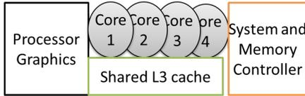
Figure 4: Intel core i7 Ivybridge architecture for parallel computing.
