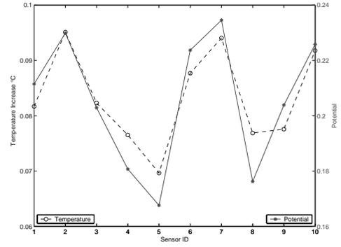
Fig. 7. Temperature Increase Potential (TIP) predicts the trend of temperature increase. High TIP results in high temperature increase, or vice versa.
