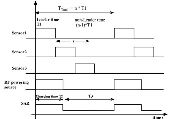
Fig. 2. Working period of sensors, cluster leader is rotated every  $T_1$  units of time.
