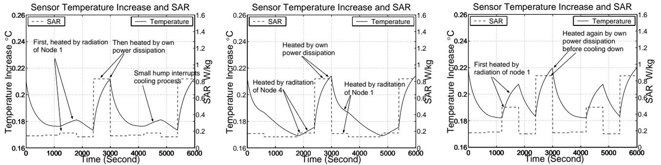
(a) Ideal Rotation Sequence of Fig 3(a) with Peak Value  $0.212^\circ C$  and Lowest Value  $0.174^\circ C$ .
