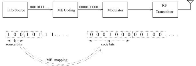
Fig. 2. Block Diagram of ME Mapping Scheme
