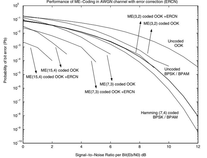
Fig. 7. Performance of Me-Coding with Error Correction
