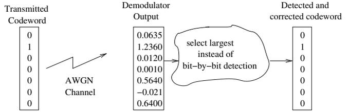
Fig. 6. Error Correction with Code-by-Code Detection
