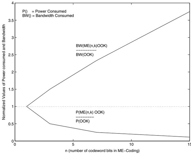
Fig. 5. Normalized Bandwidth and Power Consumption
