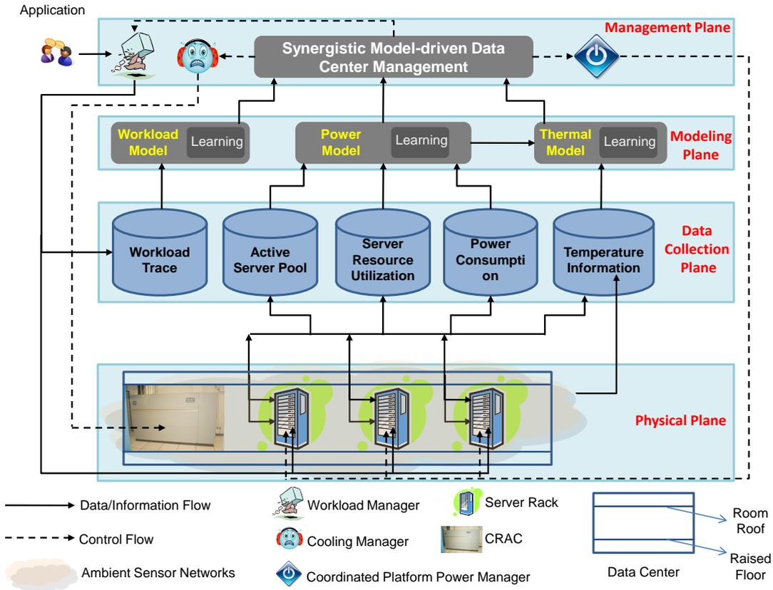
Fig. 4. Model-driven Management Architecture for Data Centers
