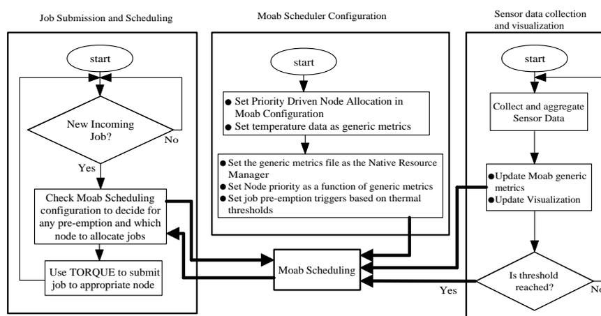
Fig. 15. Three principal modules for the thermal aware scheduler. The thick arrows are used to depict how different modules affect the Moab scheduling and vice versa.
