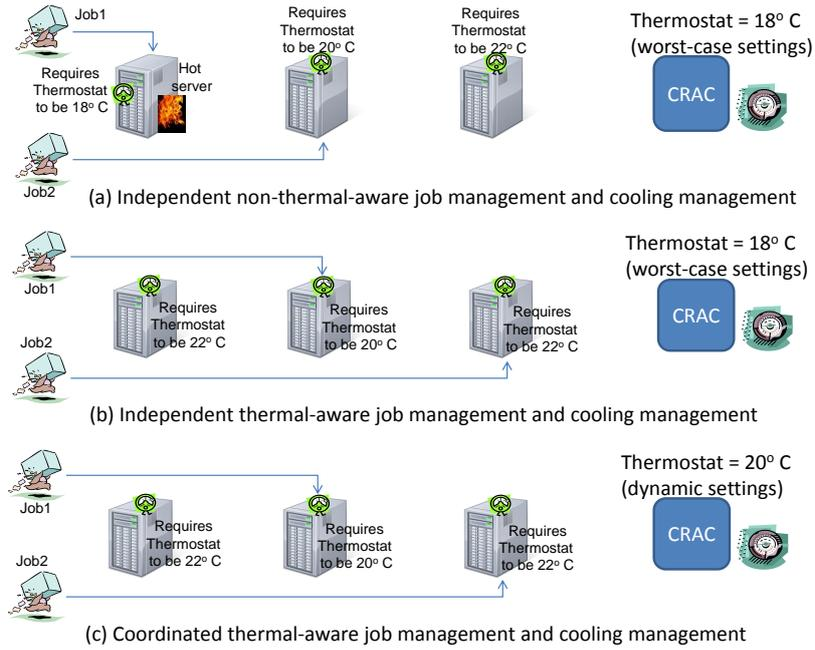
Fig. 2. Example of data center management for three servers and two jobs where the first (i.e. the left-most) server can create hot-spot if a job is assigned to it. Integrated job management and cooling management can enable higher CRAC thermostat settings (to reduce cooling energy consumption).
