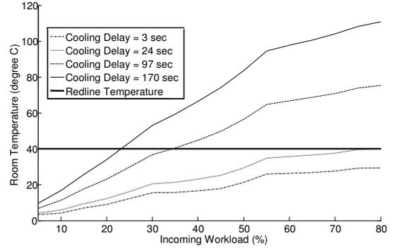
Fig. 12. Variation of ambient temperature for different cooling delay w.r.t. incoming workload in the ASU HPC data center.
