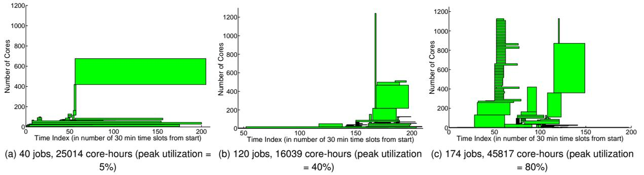
Fig. 7. Two-dimensional Gantt-like plots of three submission log snapshots of the ASU HPC data center used as simulation scenarios. Each job is depicted as a rectangle with the arrival time as the abscissa of its lower left corner, the estimated execution time as its length, and the requested numbers of processors as its height (source: [9]).
