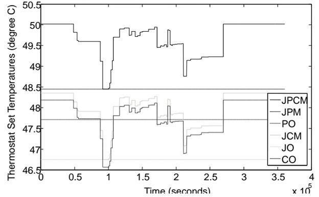
Fig. 9. CRAC thermostat set temperatures with respect to time when different management policies are employed (peak utilization = 80%, as shown in Figure 7(c)).
