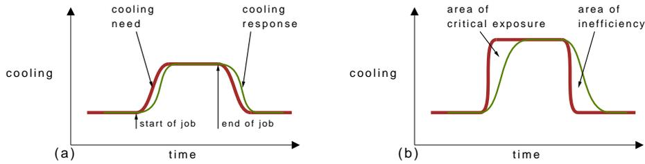
Fig. 1. Conceptual plots of the cooling delay problem. (a) A reference plot for medium density data center: the thick line shows the need for cooling while the thinner line shows the cooling supply; the supply closely follows the need. (b) In highly dense data centers, the equipment heats up faster and higher; however, the cooling technology is still as slow to respond, creating windows of critical heat exposure and of inefficiency.
