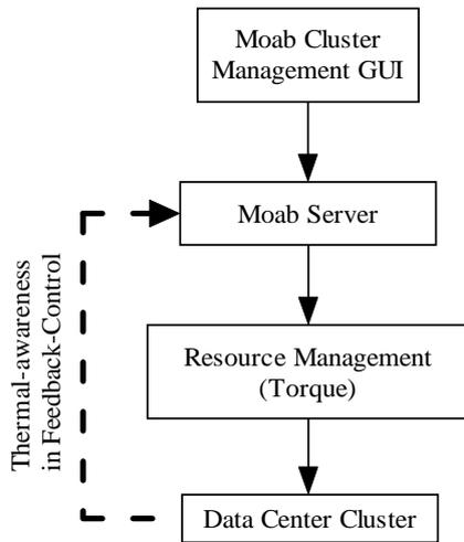
Fig. 13. Software structure of Moab.
