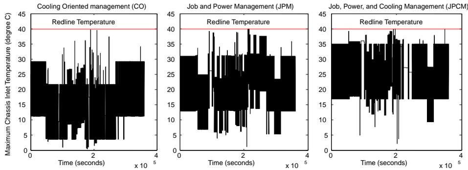
Fig. 10. Maximum chassis inlet temperature for 80 % utilization under linear cooling model for different energy management policies. Only CM, JPM, and JPCM as representative of non-coordinated cooling, no cooling management, coordinated cooling management, respectively. JPCM allows highest maximum inlet temperatures (without violating the redline) among all the policies.
