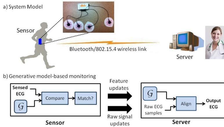
**Figure 1: a) System model for the generative model-based ECG monitoring system. A SHIMMER 2R mote is used as the ECG sensor and a PC is used as the server. b) Illustration of the generative model-based monitoring scheme.**
