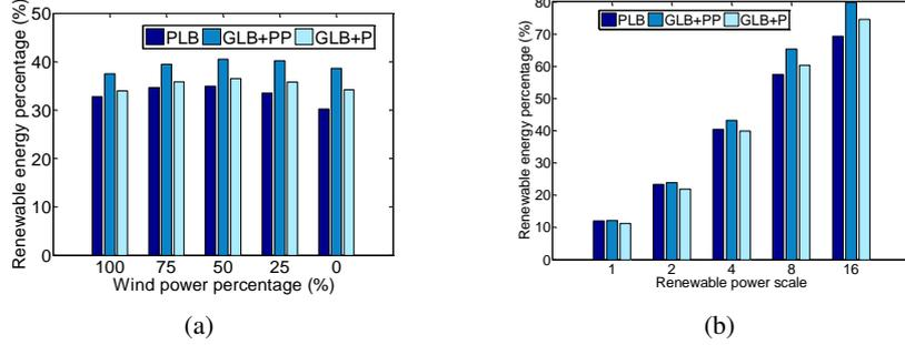
**Fig. 10.** (a) Renewable energy percentage of total energy consumption versus various mix of wind and solar energy, and (b) Renewable energy percentage of total energy for homogeneous DCs versus increase in available renewable.
