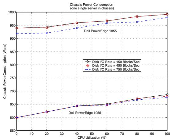
Fig. 1. Chassis Power Consumption for Single Server in Chassis.
