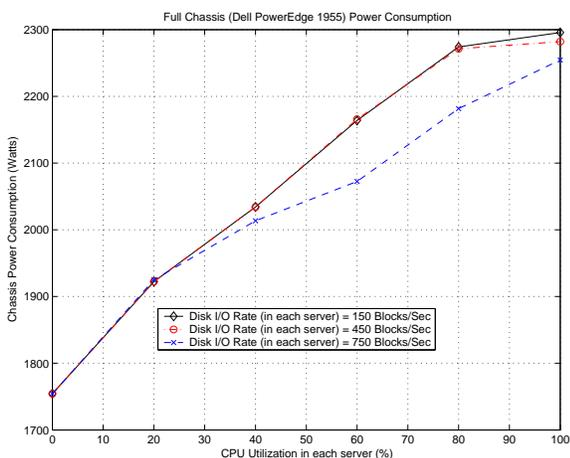
Fig. 2. Dell PowerEdge 1955 Full Chassis Power Consumption.
