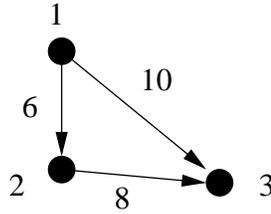
Figure 2: A topology of wireless network with 3 nodes where node 1 is the source node. The figure shows all the existing wireless links. Labels associated with the edges are the average energy cost of a node for transmitting packets over the link, such as energy cost for node 1 transmitting packet to node 2 is 6 EU/packet. Assume the residual battery energy at all three nodes is 200 EU.
