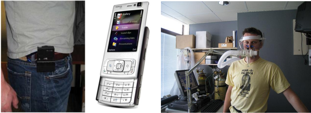
Figure 1. Photographs of the system hardware. (left) The Mobile Sensing Platform (MSP) shown worn on the hip. (middle) The Nokia N95 mobile phone. (right) Test subject wearing apparatus attached to a metabolic cart for measuring oxygen consumption during treadmill testing.
